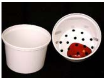
This cup, with holes, allows the lens to be immersed into the dye without any clamp
