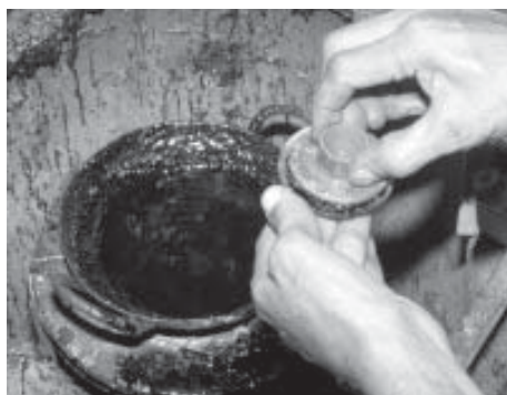
Fig. 5.17- Blocking with heated pitch
